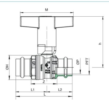
The Buna O-ring is fitted to the stem of the valve as the best possible protection against potential gas leakage under extreme duty, or low pressure applications. A secondary P.T.F.E stem seal will also assure that the valve is suitable for use up to 366°F.
