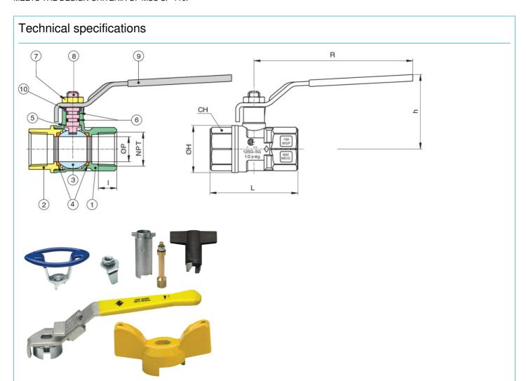
The Buna O-ring is fitted to the stem of the valve as the best possible protection against potential gas leakage under extreme duty, or low pressure applications. A secondary PTFE stem seal will also assure that the valve is suitable for use up to 366°F.
