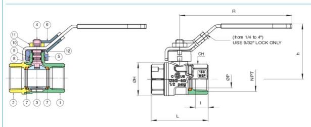
The Buna O-ring is fitted to the stem of the valve as the best possible protection against potential gas leakage under extreme duty, or low pressure applications. A secondary PTFE stem seal will also assure that the valve is suitable for use up to 366°F.
