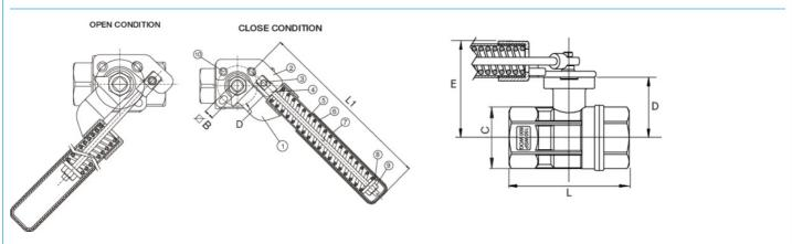
The Buna O-ring is fitted to the stem of the valve as the best possible protection against potential gas leakage underextreme duty or low pressure applications.
