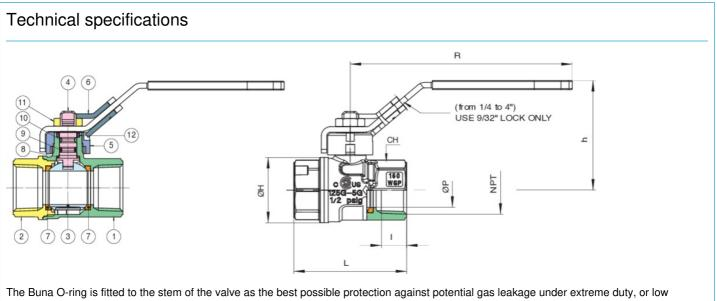
pressure applications. A secondary P.T.F.E stem seal will also assure that the valve is suitable for use up to 366°F.
