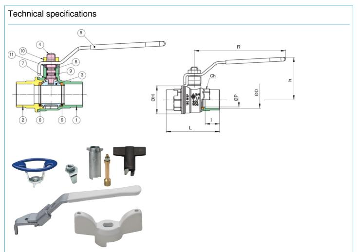
The Buna O-ring is fitted to the stem of the valve as the best possible protection against potential gas leakage under extreme duty, or low pressure applications. A secondary P.T.F.E stem seal will also assure that the valve is suitable for use up to 366°F.
