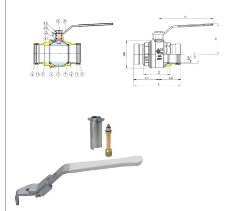
The Buna O-ring is fitted to the stem of the valve as the best possible protection against potential gas leakage under extreme duty, or low pressure applications. A secondary P.T.F.E stem seal will also assure that the valve is suitable for use up to 366°F.
