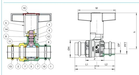
The Buna O-ring is fitted to the stem of the valve as the best possible protection against potential gas leakage under extreme duty, or low pressure applications. A secondary P.T.F.E stem seal will also assure that the valve is suitable for use up to 366°F.
