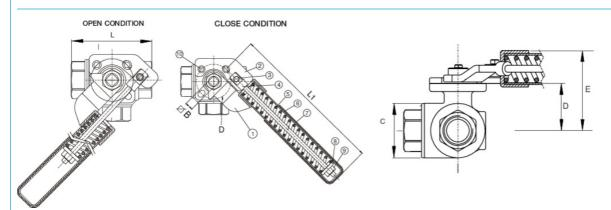
The Buna O-ring is fitted to the stem of the valve as the best possible protection against potential gas leakage under extreme duty, or low pressure applications. A secondary P.T.F.E stem seal will also assure that the valve is suitable for use up to 366°F.
